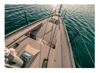
We put a lot of emphasis on a clean deck. This was realized with the "X-Brace", which functions as a canopy, halyard cover and aero element
